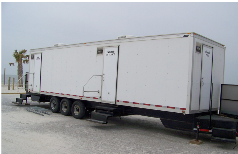
This mobile rest room does not meet ADA requirements.
